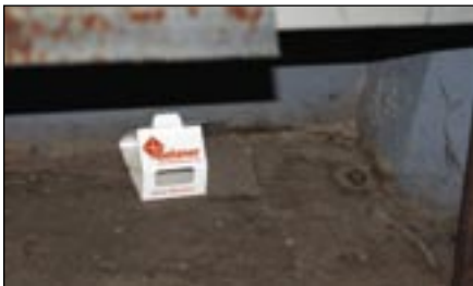
Figure 1. Floor/wall junctions are good locations for monitor placement.
